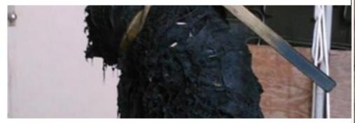
The system had to send in the divers nearly 100 feet (30 meters) into a sewer well after the wipes, congealed by grease and other items sent into the pipes, clogged the suction intake pumps to the Plum Island Wastewater Treatment Center on James Island.
